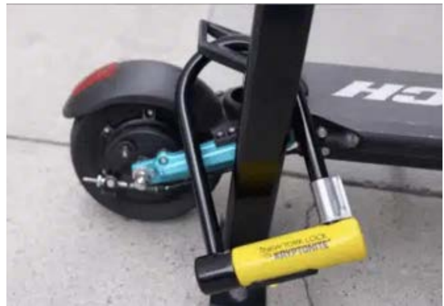
When locking an e-scooter, it is important to thread the lock through a non-removable part of the device. (riderguide.com)
