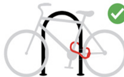
Cable lock secures rear wheel and frame.
